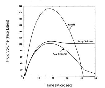
Figure 4. Volume of fluid displacement in the front and rear channel of the transducer and the bubble volume as a function of time calculated using a 3D model.
