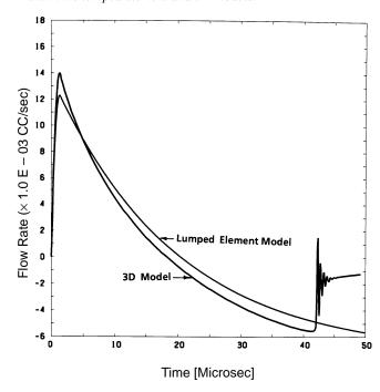
Figure 7. Flow rate in the rear channel obtained from the lumped element and 3D models.
