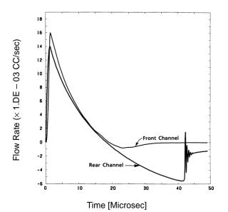
Figure 3. Flow rates in the front and rear channels of the transducer obtained from a full 3D calculation.
