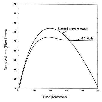
Figure 6. Comparison of front channel fluid volume displacement in the lumped element and 3D models.
