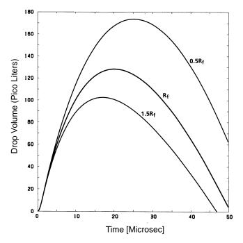
Figure 9. Fluid volume displacement in the front channel for three values of resistance.
