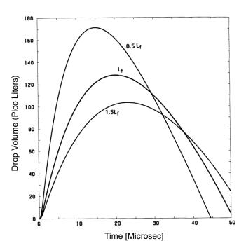
*Figure 8. Fluid volume displacement in the front channel for three values of inertance.*
