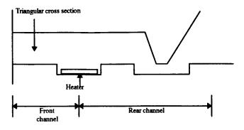
Figure 1. A channel geometry for a TIJ printhead.
